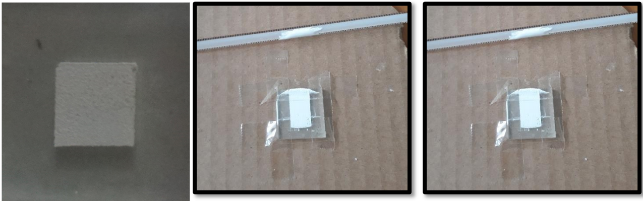
Fig. 2. Paste depositions with the doctor blade method.
